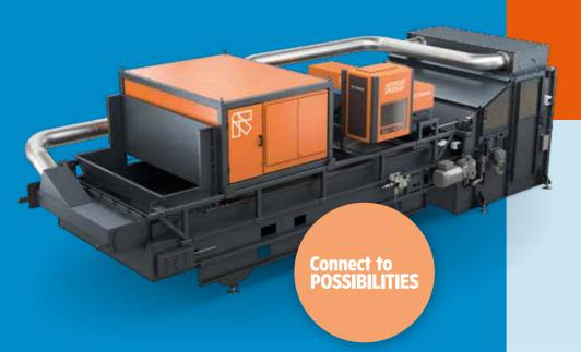
Light materials often don't lie still and are hard to detect when transported on high-speed conveyor belts. With the new AUTOSORT™ SPEEDAIR add-on for AUTOSORT™ machines, fan-driven air inlets generate a steady stream of air above the rapidly moving conveyor belt to stabilize light materials, making it easier to identify fractions. Reducing material movement on a fast-moving conveyor belt moving thus brings higher throughput rates and purity levels.
