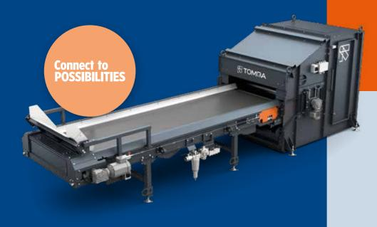
FINDER™ dominates in sorting high purity fractions regardless of the materials complexity or grain size. Utilizing patented technologies, FINDER™ detects metal objects with ultra-precision, resulting in exceptionally high yields and purity levels. Ultra-flexible thanks to its modular design, the machine is applied for various mixed waste streams and metal applications.
